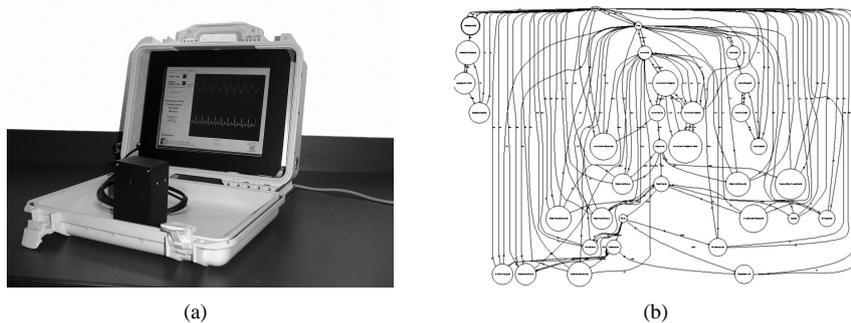
**Figure 3.** (a) The PAC simulator running on a prototype SimPod. (b) A visual representation of a FA for a sample scenario.
