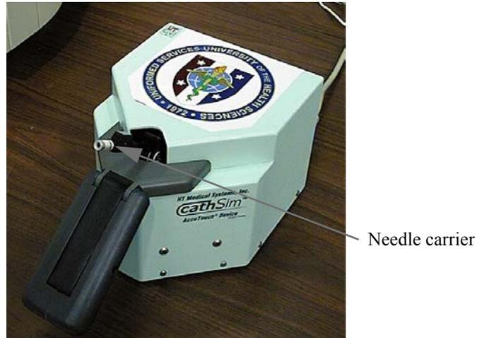
Fig. 1: Haptic interface device.
