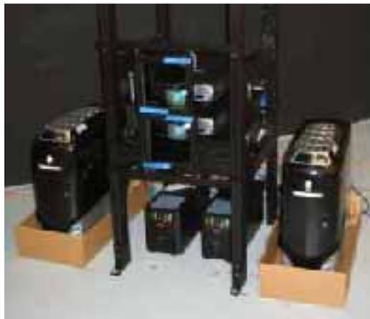
**Figure 2.** Projectors with polarized filters for stereoscopic display.
